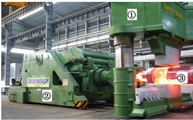
Fig. 1 An open-die forging process with huge manipulator (① Press; ② Manipulator; ③ Heavy forging)
